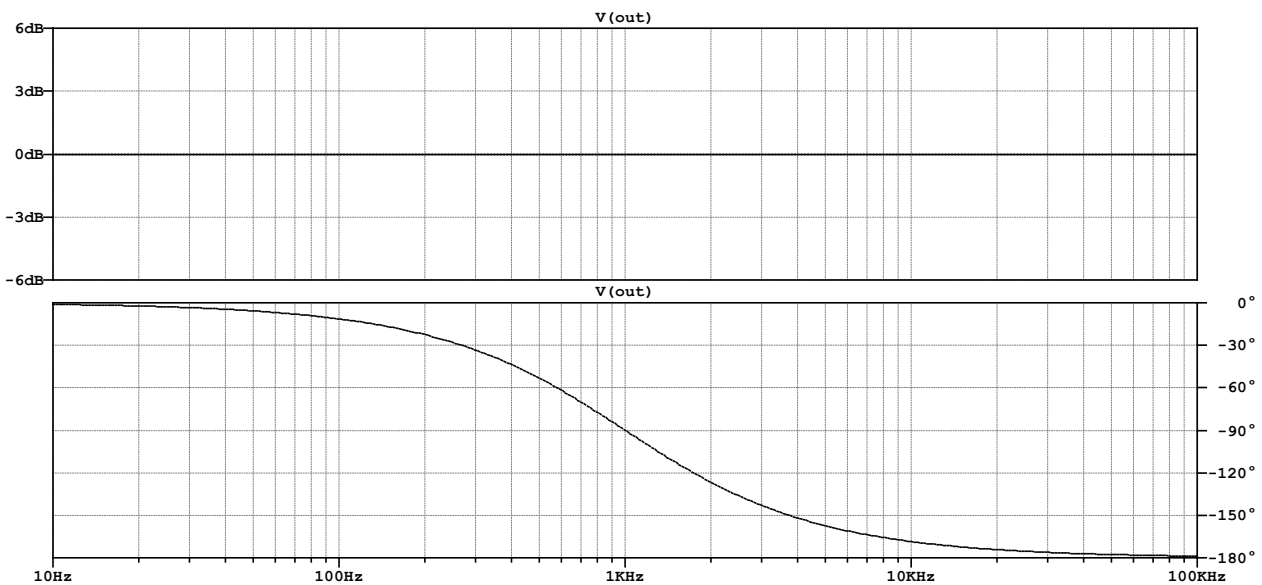
Figure 10: Bode Plots of the Single-Pole All-Pass Filter Stage
